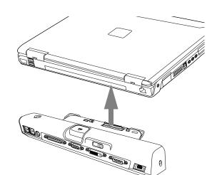
Figure 4-13. Attaching the Port Replicator
